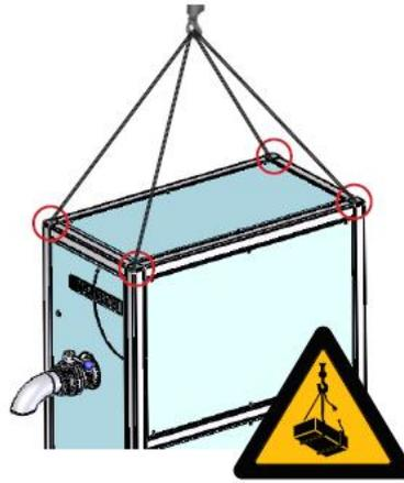
**The PR120H is supplied with thread holes for lifting eyes. Always use lifting eyes to lift the PR120H.**
